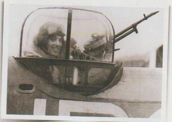
Sgt Harry Stewart in the turret of his 236 Squadron Mk.IVF at Aldergrove, September 1940, still with the single pan-fed Vickers 0.303.
