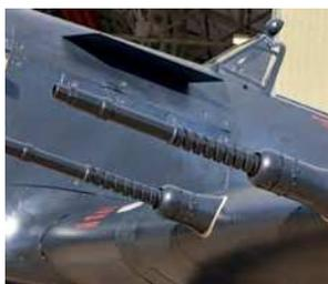
TOP: To add to the authenticity of its new night fighter intruder, BBMF Hurricane PZ865 has had exhaust shields added. These 'blinkers' were fitted to night-flying Hurricanes to prevent the pilot's vision being affected by the bright exhaust flames when flying in the dark
