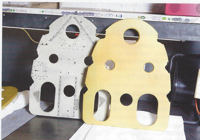
As part of the restoration, a number of new frames have been produced using the originals as a pattern. Illustrated is an old unit from the tail section assembly alongside a new component for comparison.
